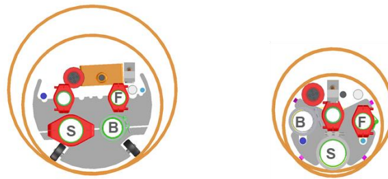
Figure 2. Pipeline cross-section for 36 / 24 inches Direct Pipe
