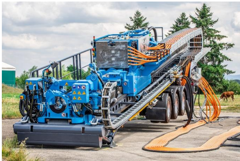
Figure 9. HK300TE: Herrenknecht's first all-electric HDD Trailer Rig with 300 ton pull force
