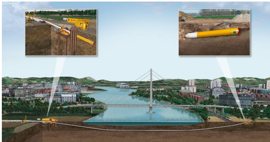
Figure 1. Functional principle of Direct Pipe for one-step pipeline installation
