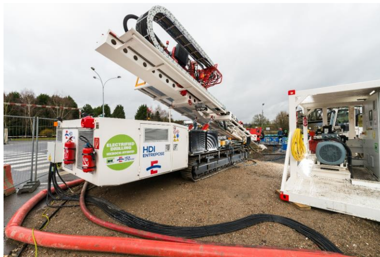
Figure 8. Herrenknecht Hybrid Rig HK80CK in operation on jobsite in France
